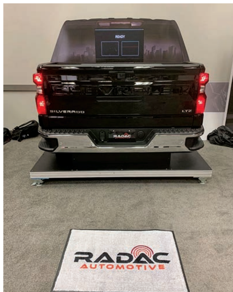
At CES, held Jan. 7-10 in Las Vegas, Radac Automotive demonstrated its millimeter wave radar module. The patent-pending technology shows how gestures can be used to open a truck tailgate hands-free.
